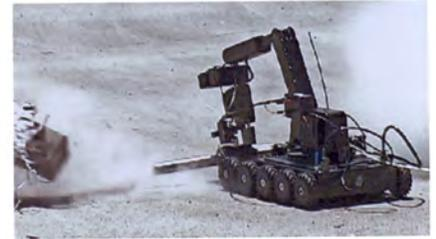
Fire disrupters at ground level from Standard Arm or 245cm elevation from Highrise Arm
