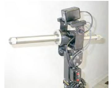
Dual-Laser Aiming Rangefinder with Camera and Firing Circuit
