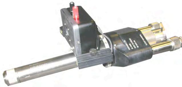
20mm caliber Recoilless Disruptor is ideally suited for firing from small robots, such as the MURV-100, at any angle and at elevations from below ground to 265cm above ground. Can also be fired from a camera tripod. Includes mounting bracket for attaching disruptor to elbow or to hand of Standard Arm. Rangefinder is extra.
