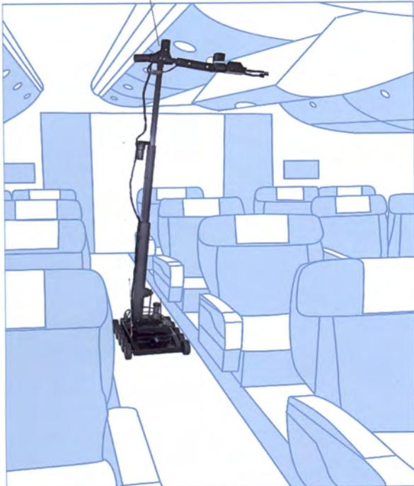
The MURV-100 can fit into narrow aircraft aisles and use the High-Rise Arm to investigate, remove or disrupt suspicious items in overhead luggage bins at heights up to 245cm (8 ft)
