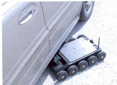
Inspect the underside of cars rapidly, directly by video, not through mirrors
